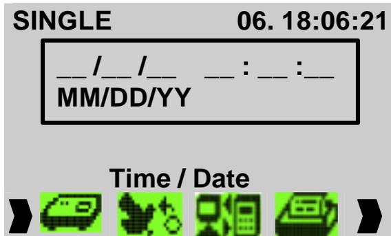
Put in date and time and press the ENTER key for confirmation and set up.
